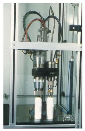
Among the various aspects of aerosol production, the gassing stage presents one of the greater hazard areas to personnel, since it involves pressurised systems. Particular care must be taken to prevent leakage and regular maintenance of all gassing equipment is essential.
